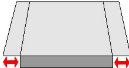
For laminates the size of the laminate usually includes an overlap and depends on whether the laminate is applied before or after edging.
